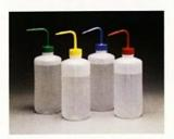
**Color-Coded Wash Bottles,** low-density polyethylene bottle; polypropylene screw closure/stem and draw tube
